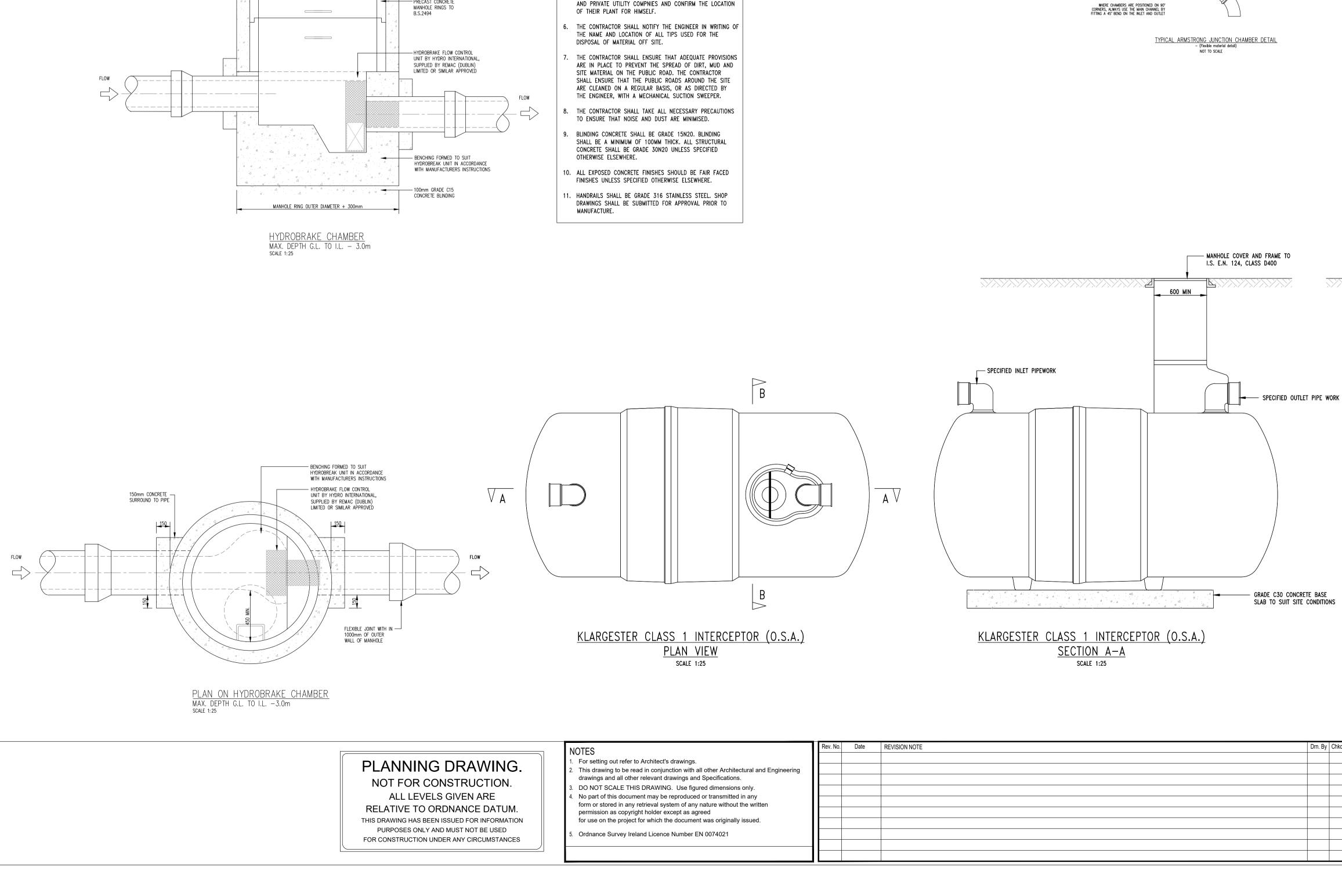
MANHOLE COVER AND FRAME TO I.S. E.N. 124, CLASS D400 600 MIN - 215mm SEMI ENGINEERING BRICK TO FINISHED LEVELS - PRECAST CONCRETE COVER SLAB TO B.S.2494  $\square$ CONCRETE SURROUND  $\begin{tabular}{ccc} \hline \end{tabular} \end{tabular}$ - LADDER RUNGS AS SPECIFIED  $\square$ - PRECAST CONCRETE
